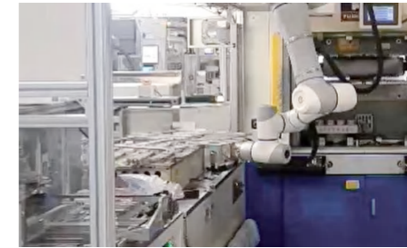
IC Packaging Loading & Unloading
